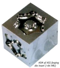
prolong the fatigue life of the die insert. This achievement minimises the need for skilled workers and the time required to polish the component in the final stage. The study results, shown in the table, demonstrate the cost savings offered by using HSM technology.
