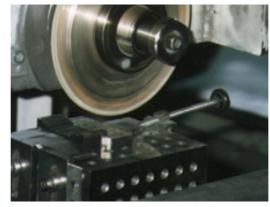
Profile grinding of a sample with GrindStar
