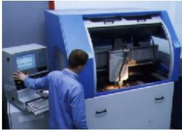
Precision abrasive water-jet cutting system
