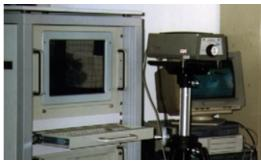
Calibration of the CNC profile grinding table with a laser interferometer
