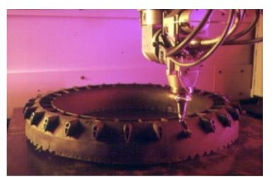
3D laser cutting for difficult-to-machine aerospace component was successfully applied
